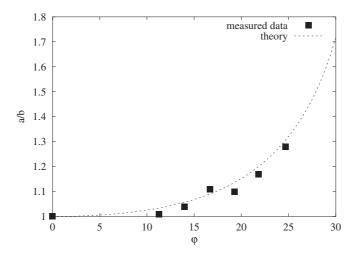
**Figure 2.** The ratio of the lattice constants a and b as a function of the tilting angle  $\varphi$  of the external magnetic field (symbols: measurements; dotted curve: calculation [9, 10]).
