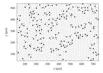
**Figure 7.** A snapshot of a liquid at  $\varphi=19^\circ$  and  $\Gamma=40$ . The number of defects is much larger than in the crystal or hexatic state (see figure 6). As expected for a liquid, there are free disclinations, though at  $\Gamma=40$  the majority are still bound in dislocations.
