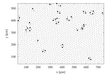
**Figure 6.** A snapshot of a sample at  $\varphi=19^\circ$  and  $\Gamma=52$  close to the melting point. Each dot represents the position of a particle, where fivefoldand sevenfold-coordinated particles are highlighted with squares and triangles, respectively.
