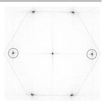
**Figure 1.** A camera image of an anisotropic colloidal crystal (left) and the corresponding Fourier transform of the particle coordinates (right). The centred rectangular structure can be recognized easily by comparing the peak positions to the vertices of a symmetric hexagon, which corresponds to a triangular lattice. The two peaks that are highlighted by circles were used to calculate the  $g_G$  correlation function.
